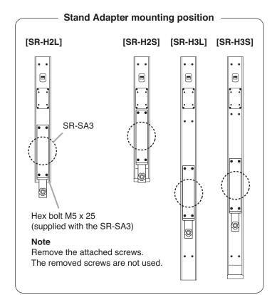
Step 2. Mount the speaker (with the Adapter attached) on the stand, then securely tighten the Adapter's knob bolt.
